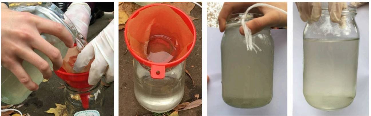
Figure 4.6. Filtration of the sample and color analysis before and after filtration.
