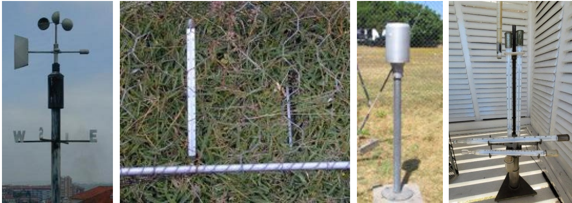
Figure 6.2. Examples of instruments deployed at meteorological station. From left to right: anemometer, grass thermometer, rain gauge, and sheltered, thermometer for maxima and minima temperature (in horizontal position) and psychrometer (in vertical position).
