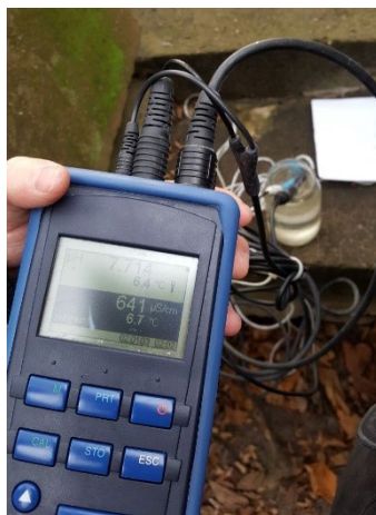
Figure 4.10. Conductivity measurement with compact precision portable meter.
