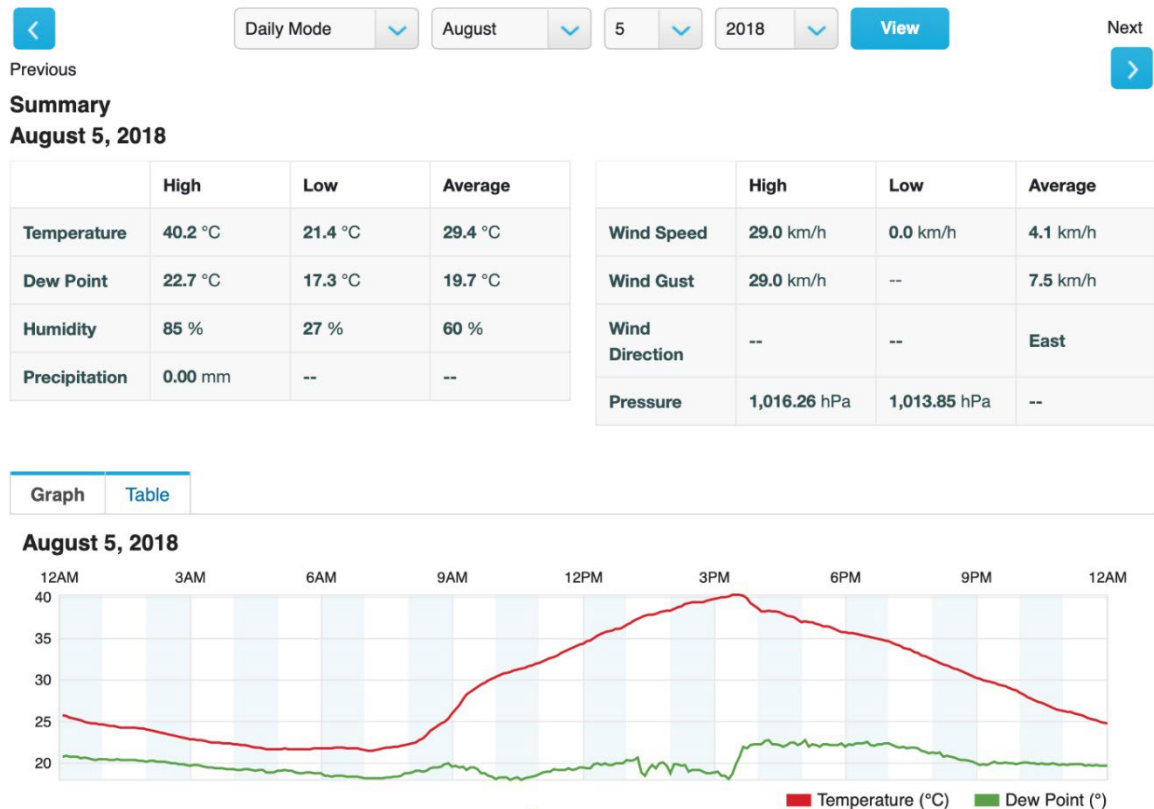
Figure 1.4. Example of an interface with weather data measured at an automatic weather station. The data were measured on August 5, 2018, at the weather station ICOIMBRA14, Portugal, coordinates 40° 11' 6"N, 8° 24' 46,8"W ( https://www.wunderground.com/dashboard/pws/ICOIMBRA14/graph/2018-08-5/2018-08-5/daily ).
