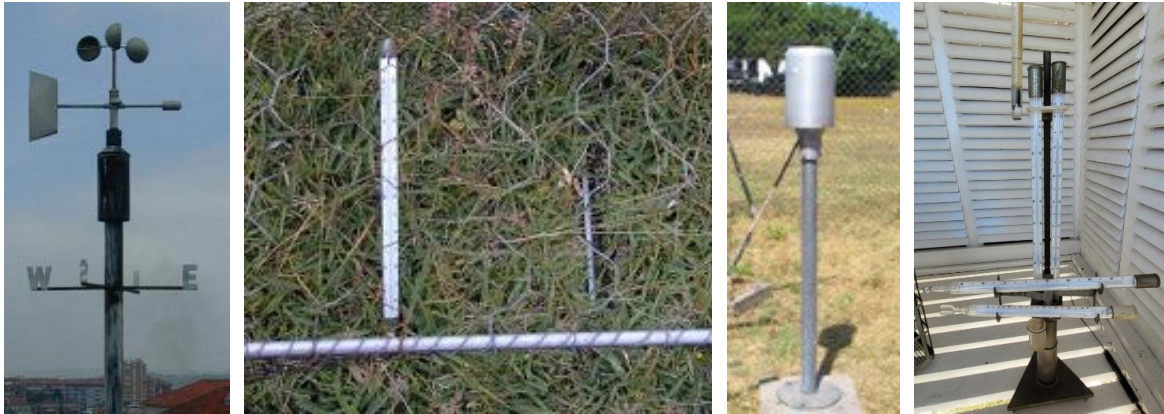
Figure 1.2. Examples of instruments deployed at meteorological station. From left to right: anemometer, grass thermometer, rain gauge, and sheltered, thermometer for maxima and minima temperature (in horizontal position) and psychrometer (in vertical position).
